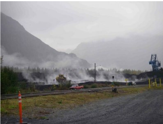
Hotspots at the Seward Coal Terminal stockpiles
