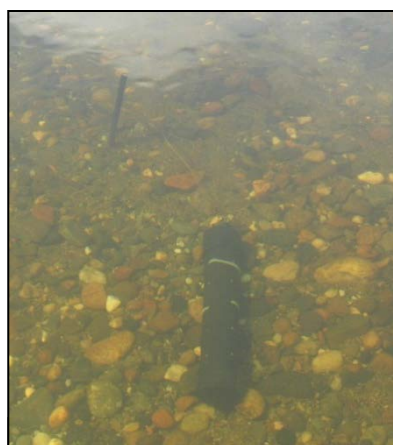
Water data logger is inside PVC housing and secured by cable to rebar.
