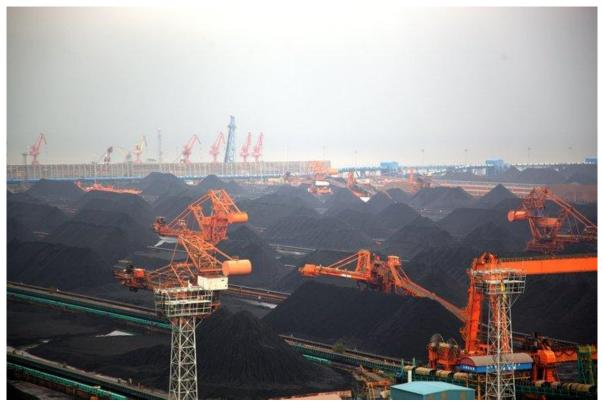
**CHINESE COAL PORT** — The crane-like stacker machines in this picture swing back and forth, and run along tracks, in order to move coal from piles onto conveyors. These conveyors are typically used to load or unload ships and rail cars. This is a standard method for handling bulk materials like coal, gravel, and ore. — Get Photo (/photos/chinese-coal-port/)
